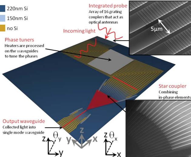
Fig. 1. Schematic of the fabricated component.
