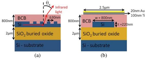
Fig. 2. Cross section of (a) grating coupler shown as the integrated probe in Fig. 1 and (b) heaters used to tune the phase as shown in Fig. 1.
